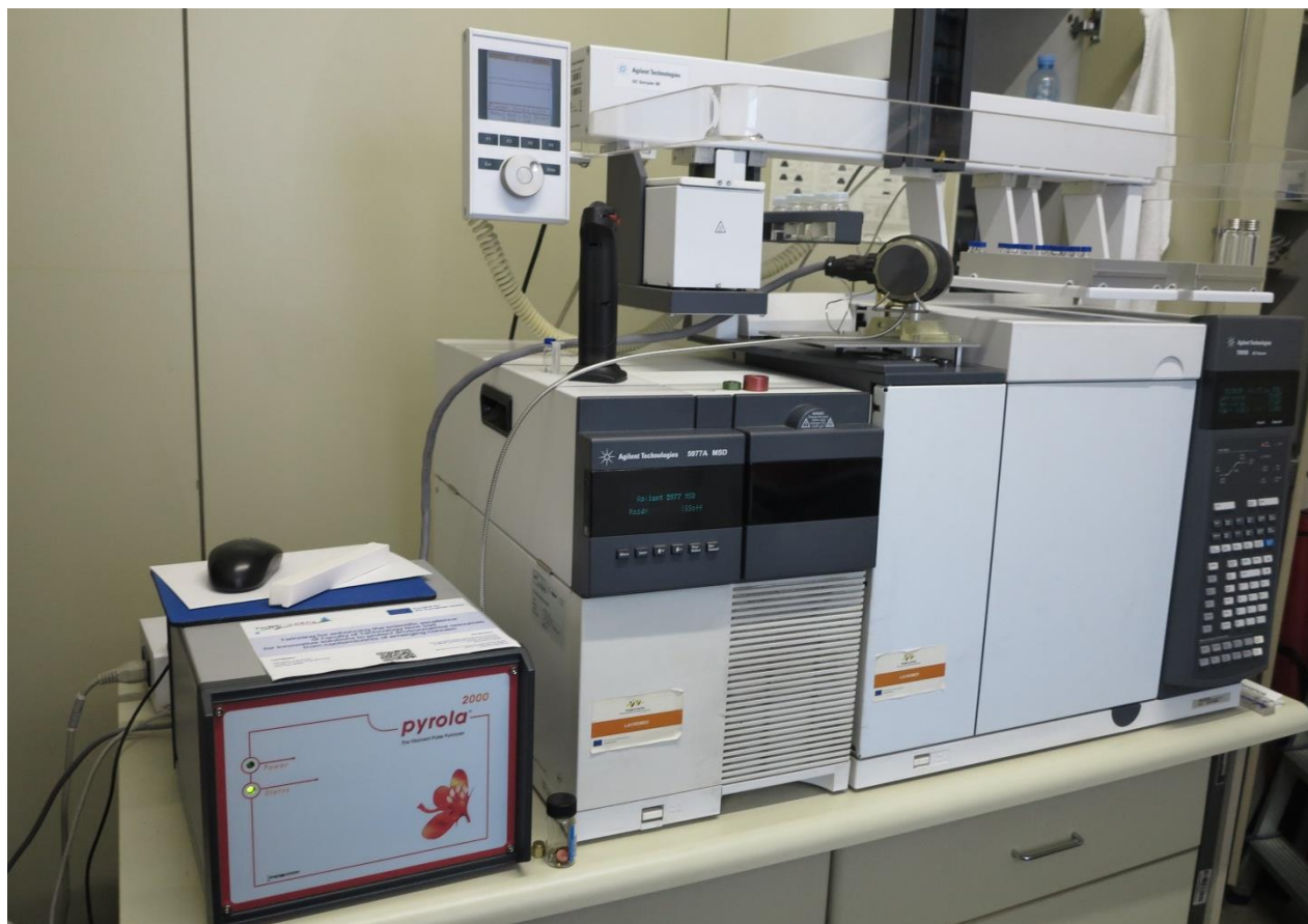
Figure 4. Pyrola 2000 process unit installed on the (top of) existing GC/MS instrument at TFNS with the Pyrola control unit (on the left) labeled with TwiNSol-CECs sticker
