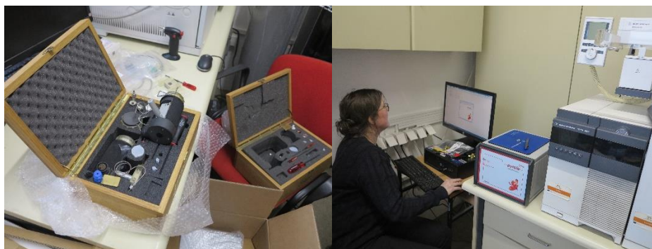
Figure 1. Pyrola® 2000 pyrolyzer (left) and its installation on GC/MS at the Lab for Chromatography at TFNS
